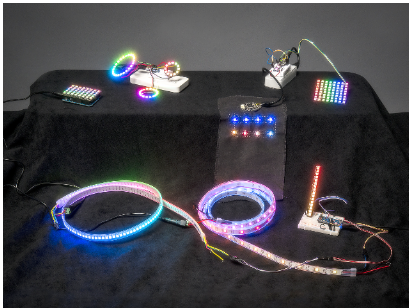
Figure 5-2. A variety of individual NeoPixels along with strips, rings, and matrices
