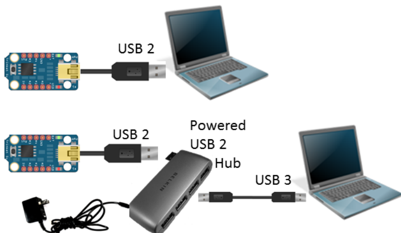
Figure 3-4. Connecting Trinket via USB 2 directly or via a USB hub
