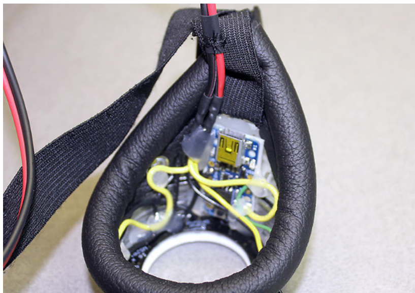
Figure 5-15. Positioning the Trinket inside the goggles
