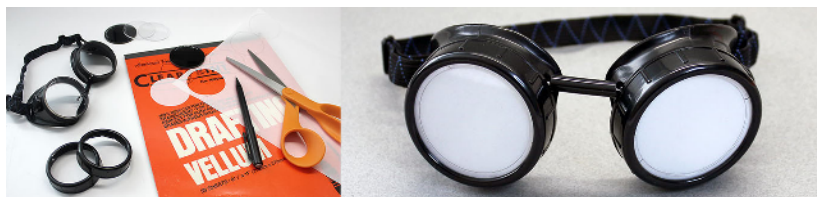
Figure 5-14. Optional vellum diffuser inserts for the goggles
