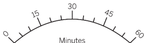
Figure 5-37. The meter face for the minutes display
