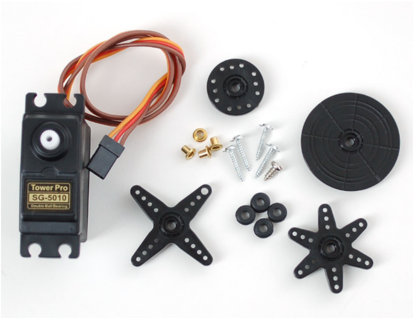
Figure 5-16. A standard servo with a variety of horns (mechanical connectors)
