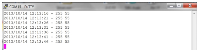
Figure 5-35. Serial output from the Analog Meter Clock software
